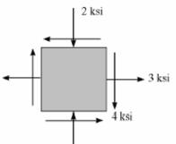
Construction of the Circle: In accordance with the sign convention,  $\sigma_x = 3$  ksi,  $\sigma_y = -2$  ksi and  $\tau_{xy} = -4$  ksi. Hence,
