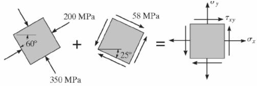
(a) with  $\theta = -30^\circ$ ,  $\sigma_{s'} = -200$  MPa,  $\sigma_{s'} = -350$  MPa
